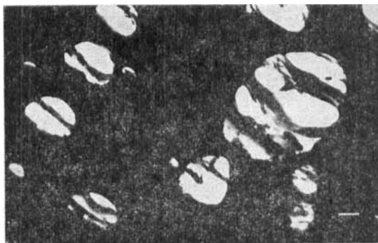
FIGURE 14 80/20 butadiene-styrene block polymer containing synthetic polyterpene resin (scale bar = 1000 nm).
